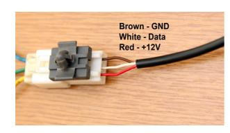
Occupation control unit placed inside passenger seat. Black cable from unit connected with car wiring installation (white connector as shown in photo, placed under the passenger seat).
